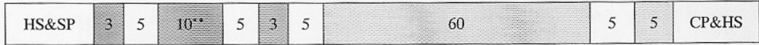
Figure 1b. Configuration of 0.25 ml straw loaded before vitrification. unit (mm); HS&SP : heat sealing & sealing powder, ■ : 25% glycerol + 25% ethylene glycol, ** : embryo column, □ : air, ■ : 0.5 M sucrose, CP&HS : cotton plug & heat sealing.
